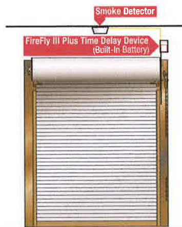
Simple-Test Fire Door System with FireFly III Plus (Built-In Battery)
