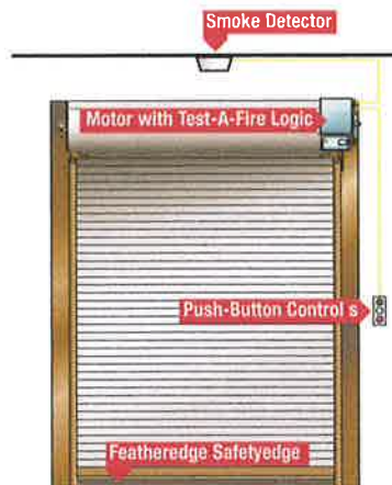
FDO-A Auto-Test Motor Operated Fire Door System
