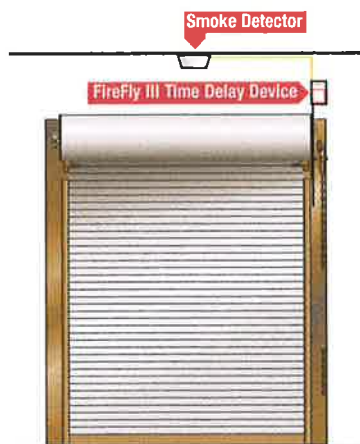
Simple-Test Fire Door System with FireFly III
